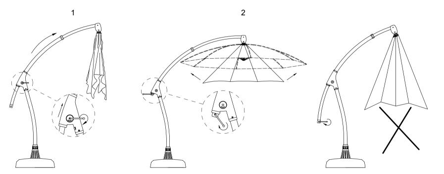
• Once the umbrella is fully opened, do not continue to turn crank, otherwise the stop mechanism will not function properly.
