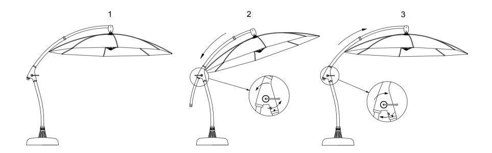
• Turn the crank counter-clockwise to tilt the umbrella to desired position when it is fully opened.
