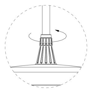
• Release the nut by turning counter-clockwise.
