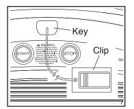
the console to be ready for use. IMPORTANT: In an emergency, the key can be pulled from the console, causing the walking belt to slow to a stop. Test the clip by carefully taking a few steps backward; if the key is not pulled from the console, adjust the position of the clip.
