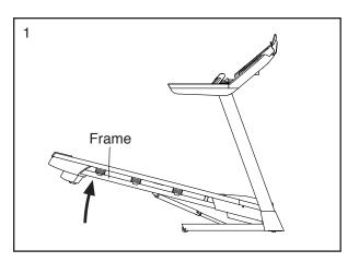
2. Raise the frame until the storage latch locks in the storage position. CAUTION: Make sure that the storage latch locks.
