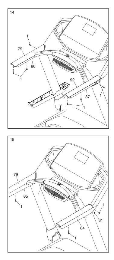
Slide the Left Bottom Handrail Cover (85) up against the Left Handrail Cover (79), and attach the Left Bottom Handrail Cover with two #8 x 1/2" Screws (1); do not overtighten the Screws.
