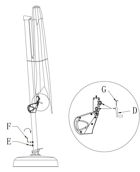
• Secure the umbrella with screws using the included allen wrench (F). Fix the crank by allen wrench (G).
