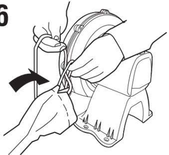
Attach longer fabric tube to blower unit making sure the tube is not twisted.
