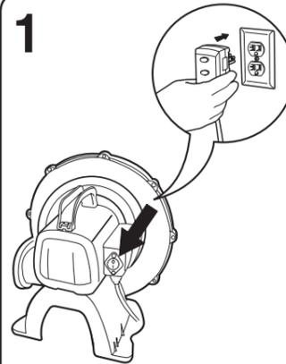
Switch power ON. If blower does not operate when switched on, press the reset button on the GFCI adaptor.
