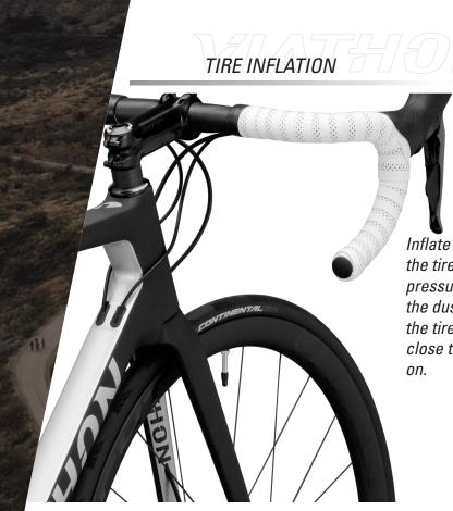
Inflate the tires. Find the marking on the tires that indicates the appropriate pressure range for those tires. Remove the dust cap and open the valve. Inflate the tire to the appropriate pressure, then close the valve and put the dust cap back
