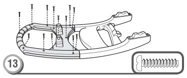
• Insert 13 - #8 x ¾" (1,9 cm) screws into the handle top and tighten.
