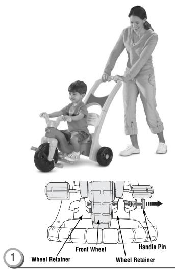
• If you are converting from the ride-on rocker mode, remove the handle pin from the wheel retainers and front wheel.
