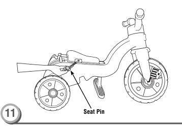
• While pushing down on the seat, insert the seat pin through the hole in the seat and into a seat mount adjustment hole.
