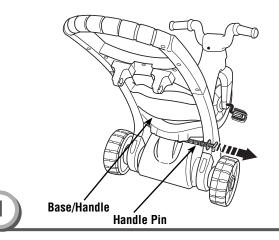
• If you are converting from the learn to pedal trike mode, remove the handle pin from the base/handle and the back of the frame.
