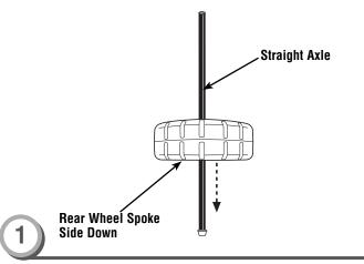
• Slide a rear wheel (spoke side down) onto the straight axle.
