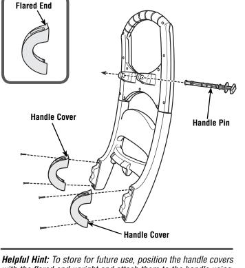
**Helpful Hint:** To store for future use, position the handle covers with the flared end upright and attach them to the handle using the four screws. Insert the handle pin into either the holes in the base/handle or through the holes in the retainers. Store the base/handle in a safe place for future use as a ride-on rocker or learn to pedal trike.
