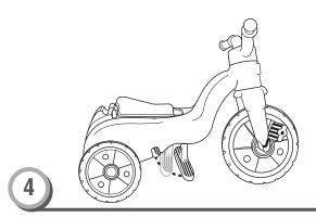
• Rotate the footrest up toward the rear wheels and snap it into the recess in the underside of the frame.
