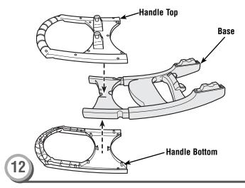
• Fit the handle top and bottom to the end of the base, as shown.
