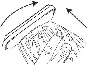
**Step 1:** Twist counterclockwise and remove the solar panel from the top of the umbrella.
