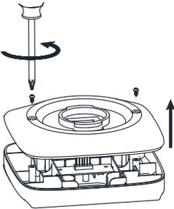
**Step 3:** Place the solar panel upside down on a flat, non-abrasive surface to avoid scratching. Remove two (2) screws on the solar panel bottom case.
