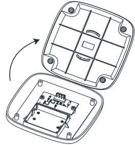
**Step 4:** Carefully open the bottom case and set aside. Replace the battery, matching the +/- on the battery with the +/- on the battery case.
