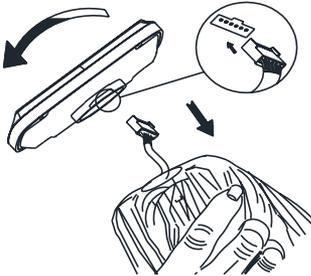
**Step 1:** Insert the plug into the socket under the solar panel.
