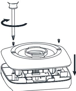
**Step 5:** Carefully put the bottom case back. Align the screw holes and replace the screws. Do not over tighten the screws.
