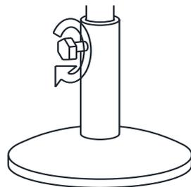
**Step 4:** We recommend that you stand and secure the umbrella to an umbrella base (not included). Secure the umbrella pole firmly by tightening the locking nut.
