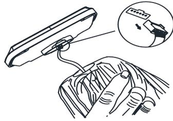
**Step 2:** Pull the plug out of the socket under the solar panel. Pull by holding the plug, not by pulling on the wires.
