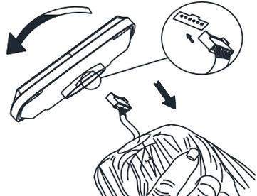
**Step 2:** Put the solar panel on the top of umbrella and hide the plug and wire inside the groove at the top of umbrella. Then turn the solar panel clockwise. Do not over tighten.
