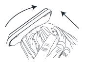
Step 1:Twist counterclockwise and remove the solar panel from the top of he umbrella.
