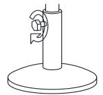
Step 3: Insert the bottom pole into the upper pole while pressing the snap button on the upper pole until the the snap button locks into position.
