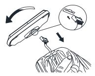
Step 1: Insert the plug into the socket under Step 2: Put the solar panel on the top of umbrella and hide the plug and wire inside the gro ove at the top of umbrella. Then turn the solar panel clockwise. Do not over tighten.
