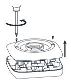
Step 3: Place the solar panel upside down Step 4: Carefully open the bottom case and on a flat, non-abrasive surface to avoid scratching. Remove two (2) screws on the the +/- on the battery with the +/- on the solar panel bottom case.
