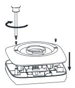
**Step 5:** Carefully put the bottom case back. Align the screw holes and replace the screws. Do not over tighten the screws.
