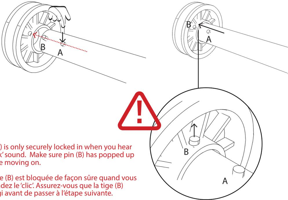
Pin (B) is only securely locked in when you hear a 'click' sound. Make sure pin (B) has popped up before moving on.
