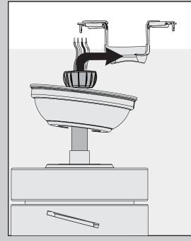
**DO NOT PICK THE FAN UP BY THE CANOPY OR WIRES.** Place the downrod ball into the slot in the ceiling bracket.
