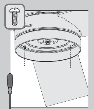
Screw two housing assembly screws from
