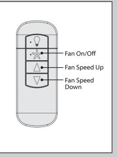
The Fan On/Off button turns the fan on or off. Adjust the fan speed using the "Fan Speed Up" or "Fan Speed Down" directional buttons.
