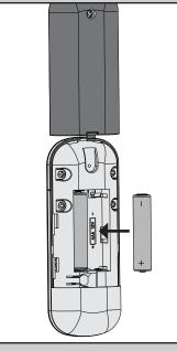
Install two AAA batteries, found in the remote control hardware bag, into the transmitter. Clean the battery contacts prior to installing the batteries. Please contact your local battery recycling center for proper battery disposal information.
