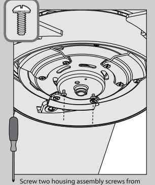
Screw two housing assembly screws from
