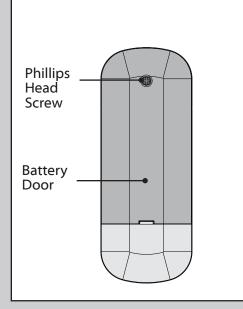
To access the battery compartment, remove the small Phillips head screw that secures the battery door to the transmitter assembly.
