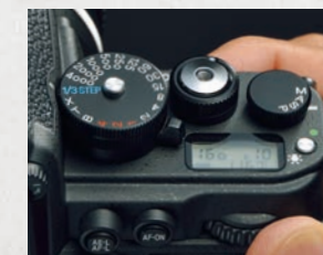
When set to 1/3 STEP, shutter speed can be controlled via the main command dial without taking your eye from the viewfinder
