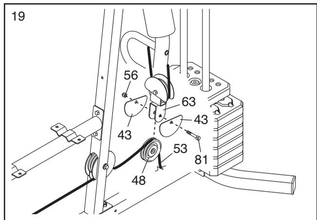
20. Route the Low Cable (53) under a 90mm Pulley (48). Attach the Pulley and two Half Guards (43) to the Base (1) with an M10 x 46mm Bolt (81) and an M10 Locknut (56). **Make sure that the Half Guards are on the outside of the bracket as shown.**
