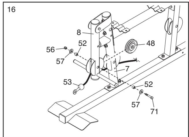
17. Attach a 90mm Pulley (48) inside the Front Leg (7), over the Low Cable (53), with an M10 x 67mm Bolt (71), two M10 Washers (57), two 12mm Spacers (52), and an M10 Locknut (56).
