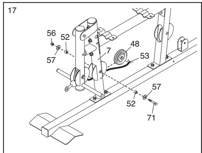
18. Route the Low Cable (53) under a 90mm Pulley (48) and through the Upright (3). Attach the Pulley inside the Upright with an M10 x 67mm Bolt (71), two M10 Washers (57), two 12mm Spacers (52), and an M10 Locknut (56).
