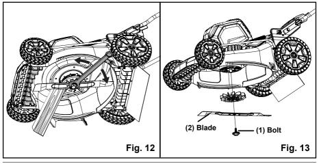
NOTE: Be sure to replace the parts in the exact order in which they were removed. When installing the cutting blade, verify that it is installed with the curved ends pointing toward the mower deck, and not toward the ground. Refer to the schematic drawing on page 30 of this manual.
