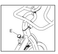
To stop the flywheel, push the resistance knob downward. The flywheel should quickly come to a complete stop.
