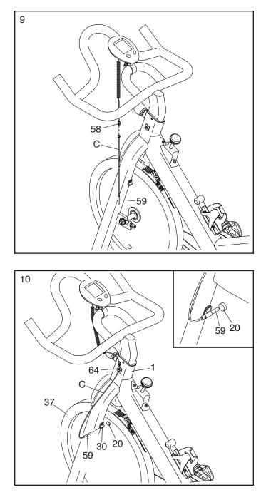
10. Insert the wire (C) on the Reed Switch (59) into the Clip (64) on the left side of the Frame (1).
