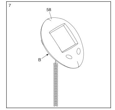
8. Slide the Console (58) onto the Console Bracket (10) on the Handlebar (7).
