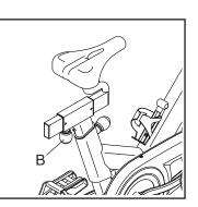
tighten the adjustment knob. Make sure that the adjustment knob is engaged in an adjustment hole.
