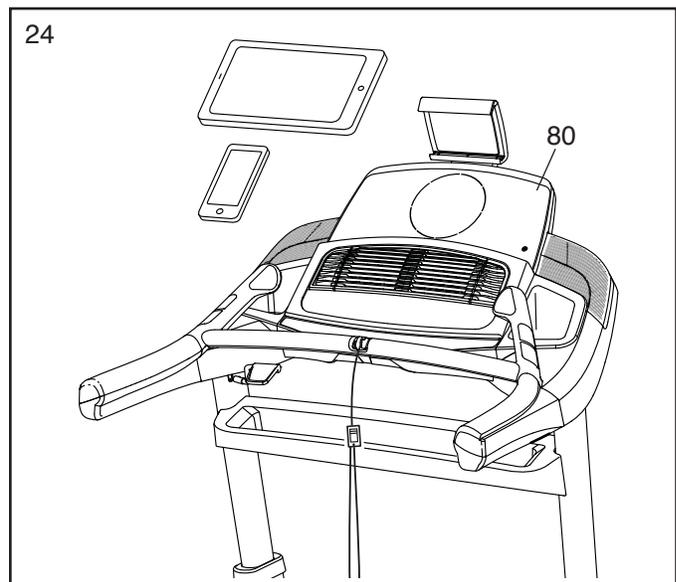
25. **Make sure that all parts are properly tightened before you use the treadmill.** If there are sheets of plastic on the treadmill decals, remove the plastic. To protect the floor or carpet, place a mat under the treadmill. To avoid damage to the console, keep the treadmill out of direct sunlight. Keep the included hex keys in a secure place; one of the hex keys is used to adjust the walking belt (see page 31). Note: Extra parts may be included.
