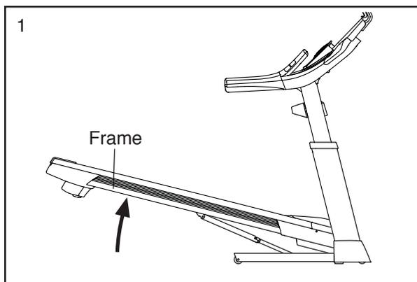
2. Raise the frame until the storage latch locks in the storage position. **CAUTION: Make sure that the storage latch locks.**
