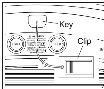
**the console to be ready for use. IMPORTANT:** In an emergency, the key can be pulled from the console, causing the walking belt to slow to a stop. Test the clip by carefully taking a few steps backward; if the key is not pulled from the console, adjust the position of the clip.
