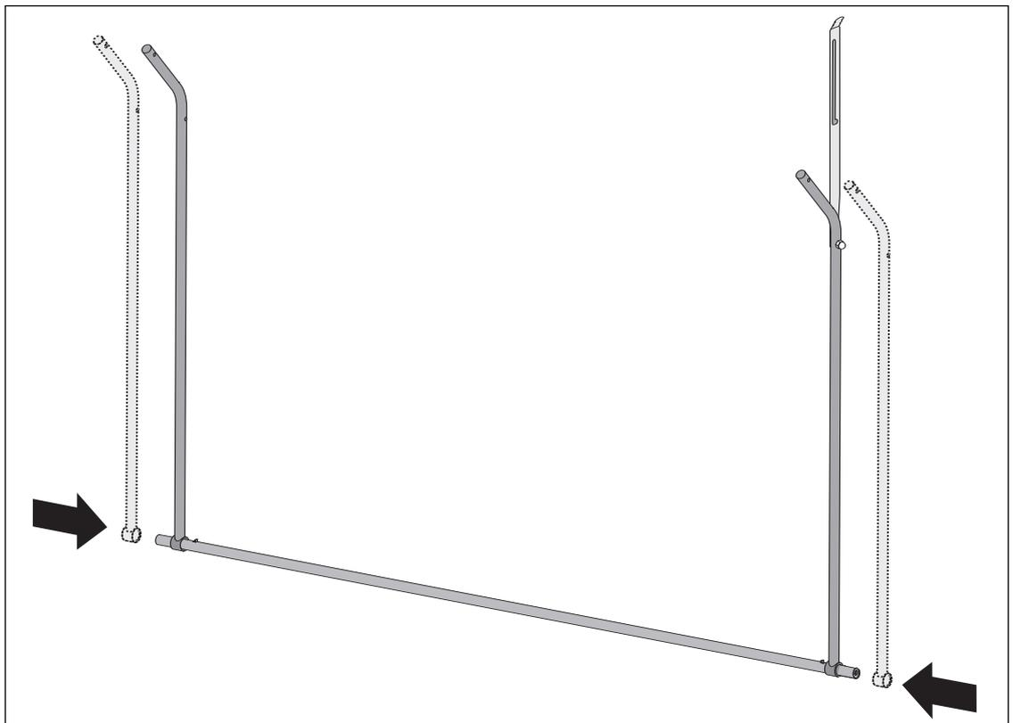
It is necessary to secure the table half against sliding and/or overturning for the following steps. First, have a second person bolt the round crossbar to the wheel base.
