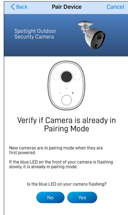
Check if the LED indicator of your camera is blinking blue slowly as shown. If so, your camera is already in pairing mode (i.e., the camera's hotspot is activated temporarily) and ready to pair. Tap the **Yes** button.
