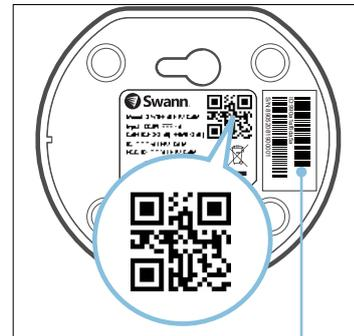
If your phone can't scan the QR code, tap the **Manual Entry** button at the bottom of the QR code scanning screen and type in the camera's ID (consists of 12 alphanumeric characters) located on this sticker label.
