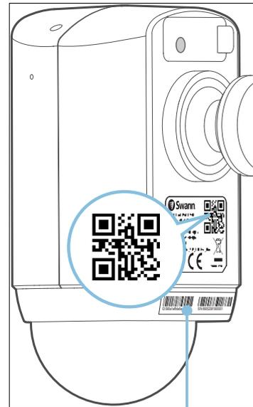
If your phone can't scan the QR code, tap the **Manual Pair** button at the bottom of the QR code scanning screen, select "Floodlight Security Camera" from the product menu, and type in the camera's ID (consists of 12 alphanumeric characters) located on this sticker label.
