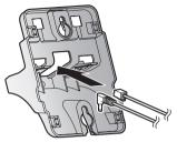
2 Tuck the telephone line cord inside the wall mounting adaptor (①). Connect the AC adaptor cord and telephone line cord (②).
